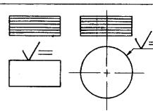
2. Perpendicular to the boundary line of the surface indicated by the symbol. Such as end view of shaping.
