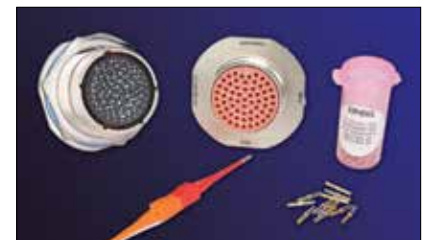
Sealed Jam Nut Receptacles (showing front and back) with Crimp Contacts - Use UTS Termination System with M39029/57 Socket Crimp Contacts and Standard Insertion/Removal Tool
