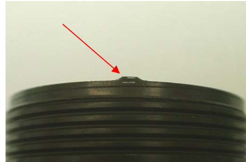
Pic 10 REJECT Majority of tooth missing
