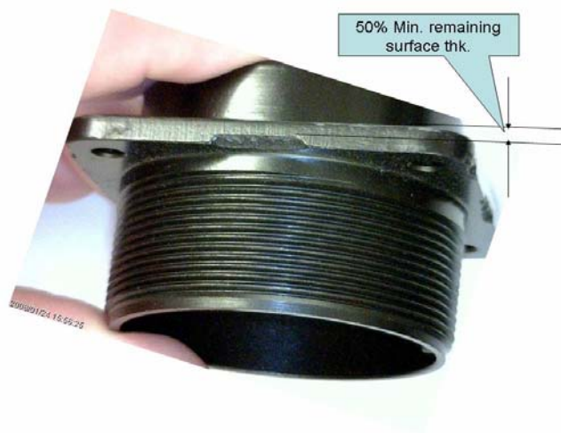
Pic 13 Gate breakage ACCEPTABLE if over 50% of material remains
