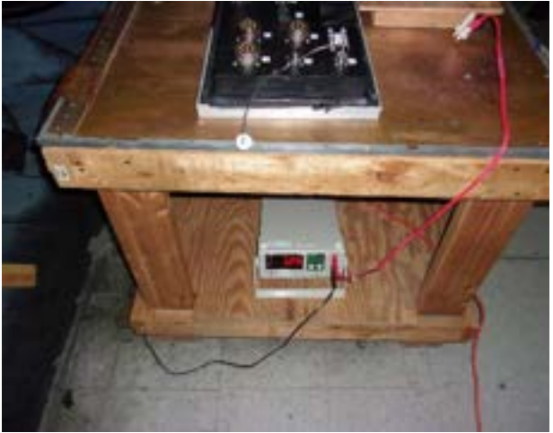
Chamber to Table Bonding Measurement
