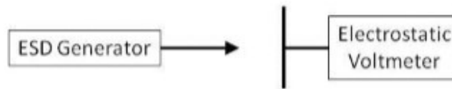
Figure 5.6-1: Measurement System Check Setup, Tip Voltage Verification
