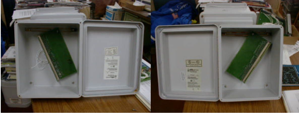
FIGURE 4. NEMA TYPE 4X ENCLOSURE USED FOR SALT ATMOSPHERE TESTING
