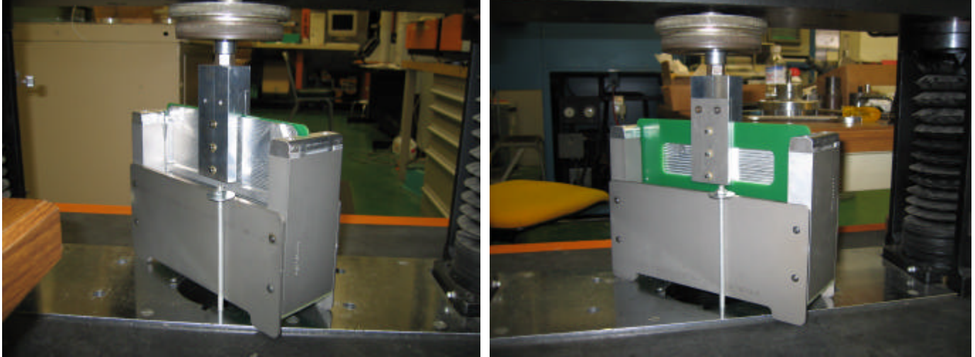
FIGURE 1. INITIAL MATING FORCE TEST SET-UP.
