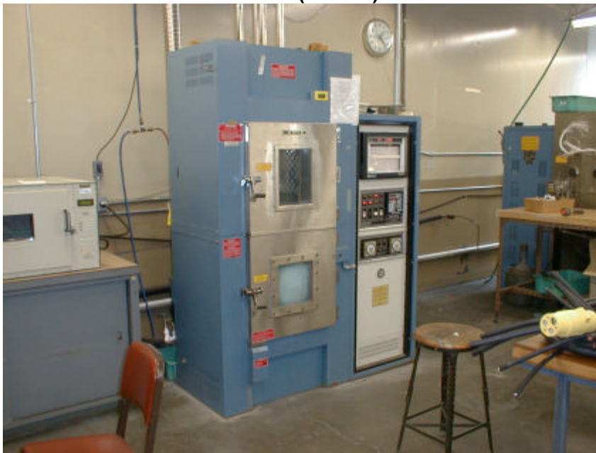
FIGURE 6. THERMAL CYCLING (SHOCK) CHAMBER
