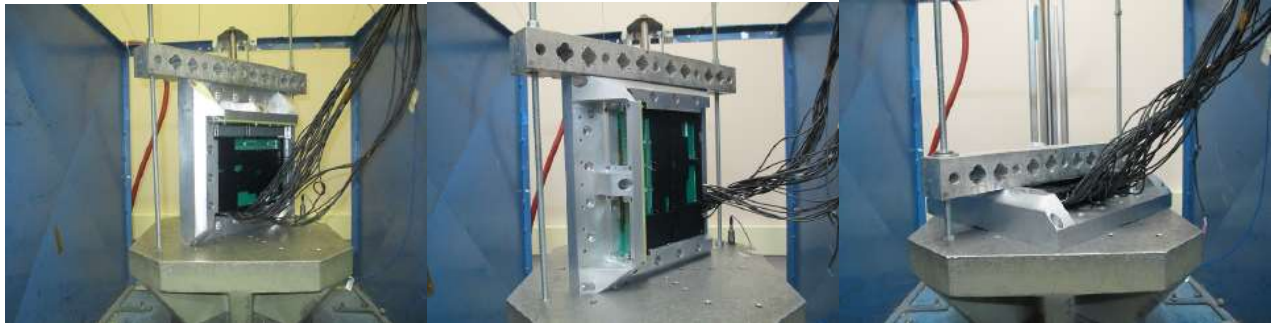
Figure 7: Mechanical Shock test set-up
