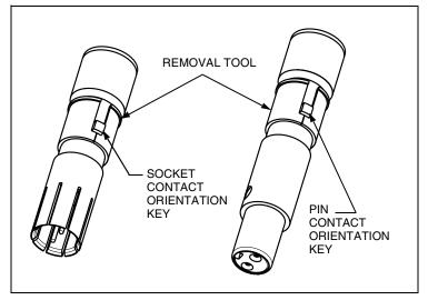
Installation Instructions (General Insertion and Removal) for Quadrax Contact Assembly for Amphenol Canada Rack and Panel Connectors.
