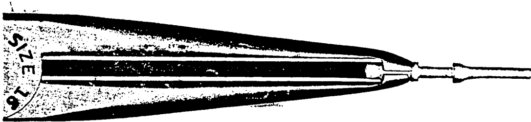
Figure 2-7. Contact Insertion Tool Positioned at Rear of Wire-well
