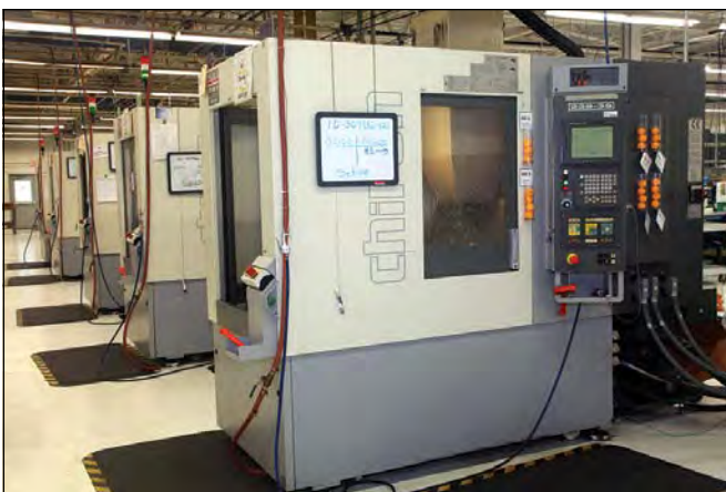
Above and below are production areas for LRM interconnects and heatsinks. Note the orange balls on the machines - these are used as a quick checking device for processes.
