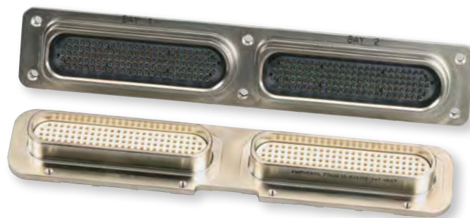
Custom 2-Bay Ruggedized, Non-Floating Brush Rack and Panel Connector (126 brush contacts per bay)
