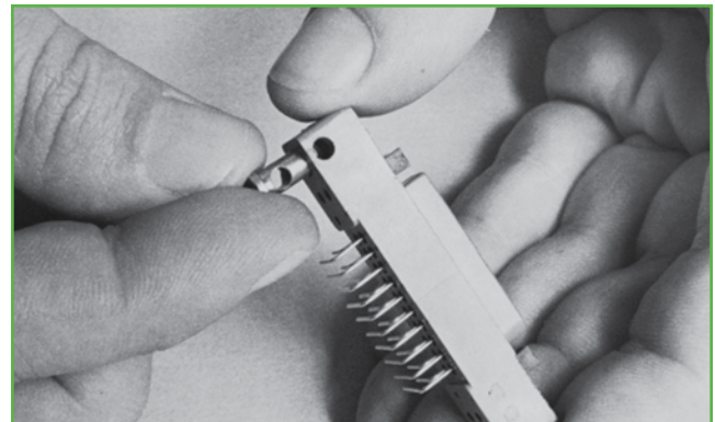
LOCKING BUSHING ACCESSORY INSERTED INTO PC CONNECTOR BODY
