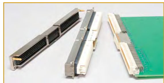
Ruggedized VME64x backplane (left), and module adapter (center) and a typical COTS VME64x circuit board (right).
