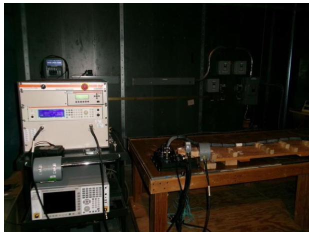
06 - CS114 Test, Power Bundle
