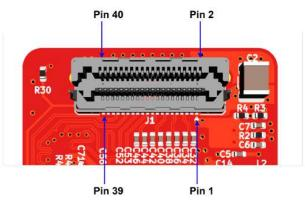
Figure 4: Razor Beam connector
