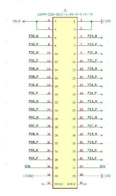
Figure 11: RAZOR BEAM connector on Daughterboards
