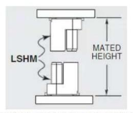
Figure 5: Razor Beam connector self-mating
