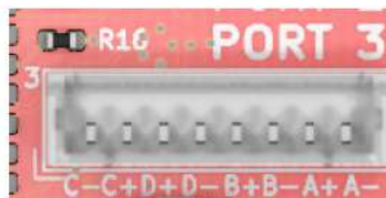
Figure 7: Mapping of ethernet signals onto PicoBlade connectors.
