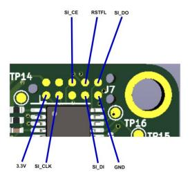
External Flash programming header pinout
