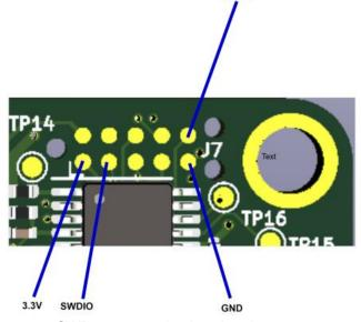
SWD programming header pinout
