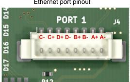
Ethernet port pinout
