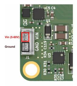
Voltage input header pinout
