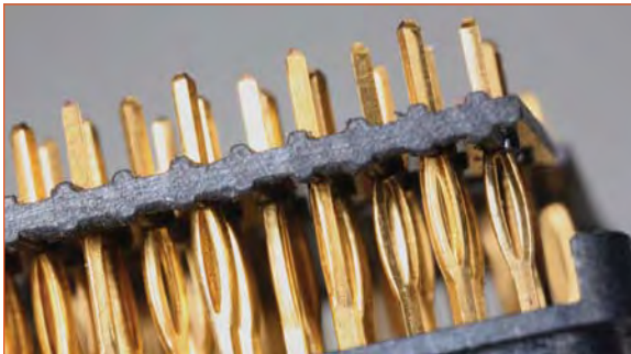
LRM backplane insert with compliant pins
