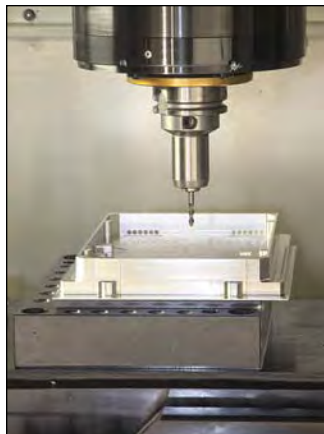
Close-up photo showing vertical machining of heatsink housings done at Amphenol.
