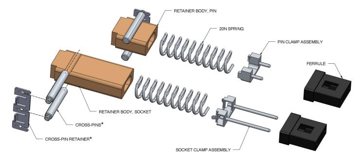
\*Cross-pins and cross-pin retainers are suppled with the base connector
