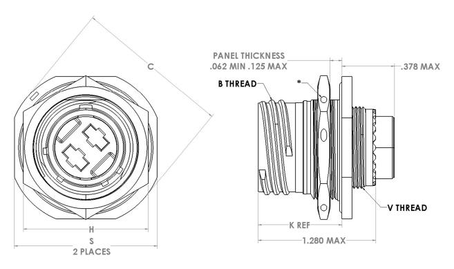
$^{\star}0.059$  dia. min., 3 lockwire holes, formed lockwire hole design (6 holes) is optional
