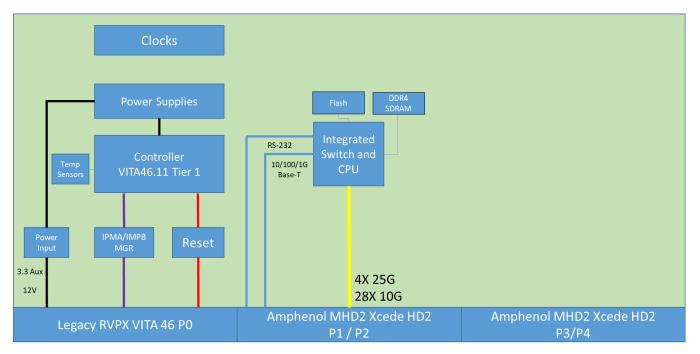
CF-02W300-17X – Single Switch – 32 channels @ 50G; Managed; 75 Watts; ~60 second boot LEGACY RVPX SOSA VARIANT
