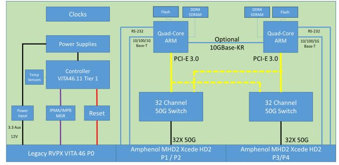
CF-02W300-13X – Dual Switch – 64 channels @ 50G; Managed; 150 Watts; ~60 second boot VITA91 SOSA VARIANT
