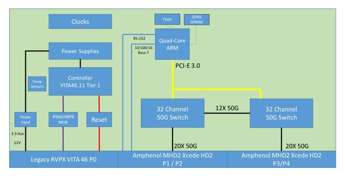
CF-02W300-15X – Dual Switch – 64 channels @ 10G/25G; Light Management; 50 Watts; ~10 second boot
