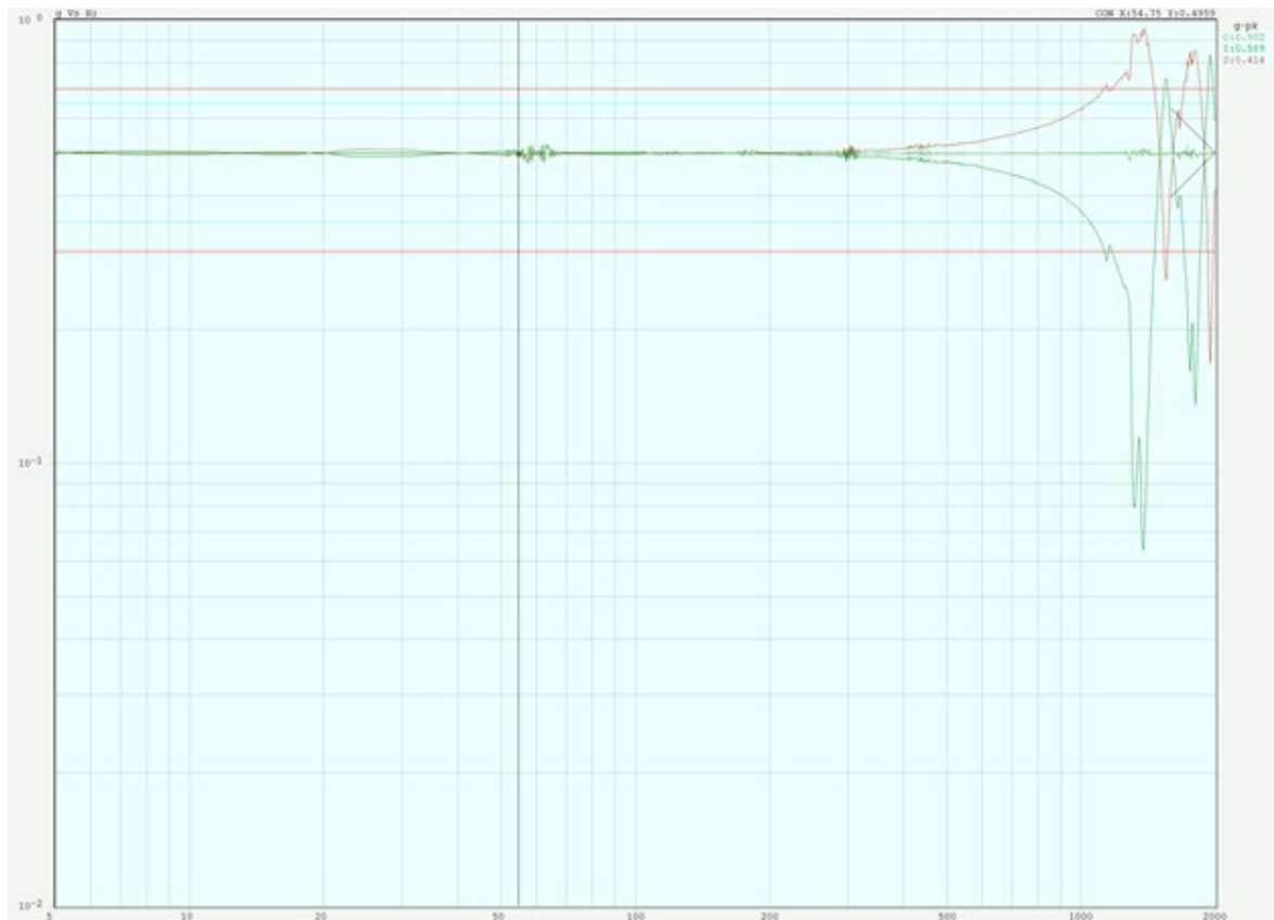
Z axis sine sweep with just the fixture
