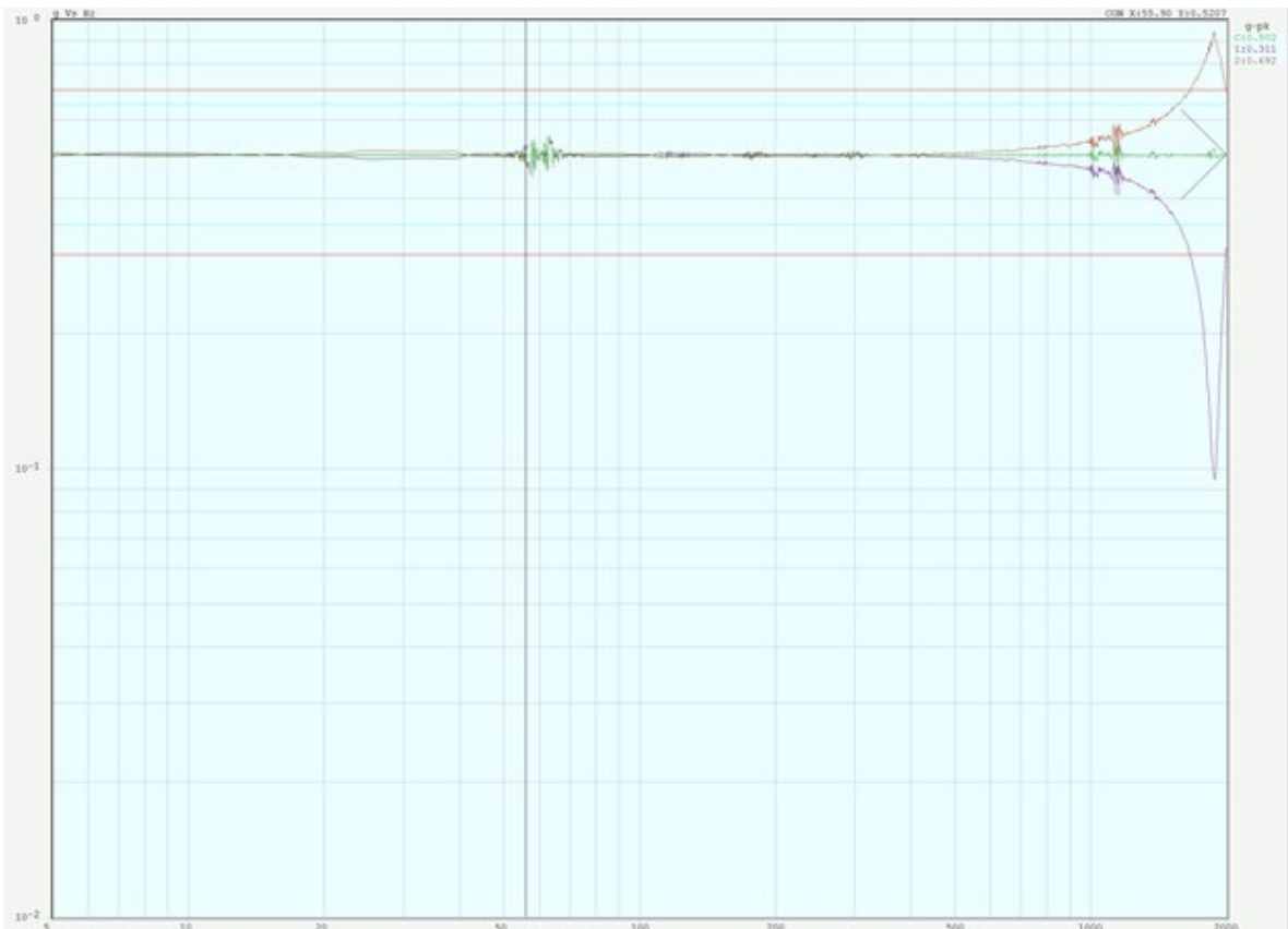
Y axis sine sweep bare fixture
