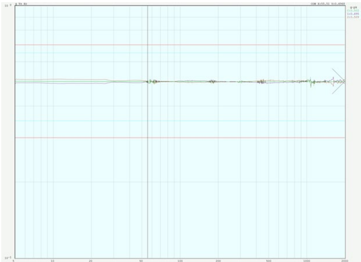
X axis Sine Sweep, Fixture, backplane and cables
