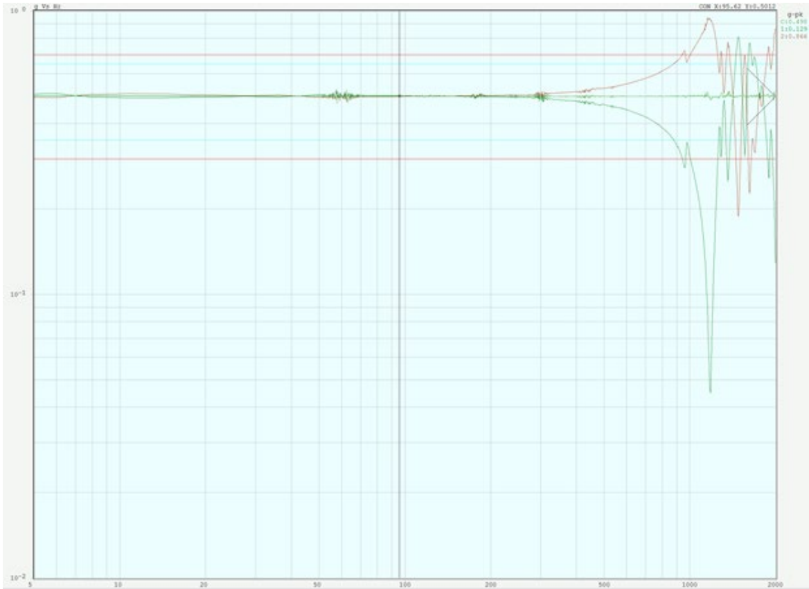
Z axis Sine Sweep with fixture and backplane
