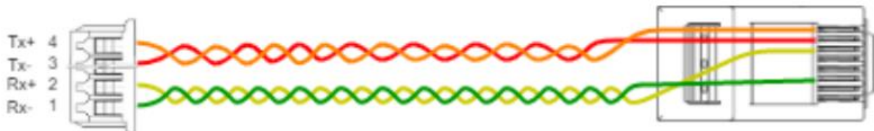
Ethernet Cable Pinout
