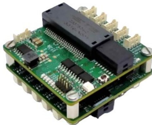
Back to Back operation (two SwitchBlox Rugged)
