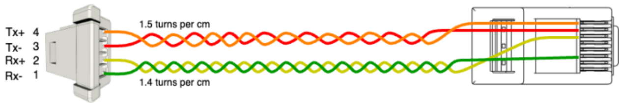
Ethernet cable pinout for Molex PicoClasp variant
