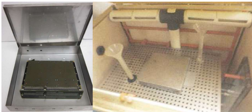
Figure 8: Salt Fog with SO 2 test set-up
