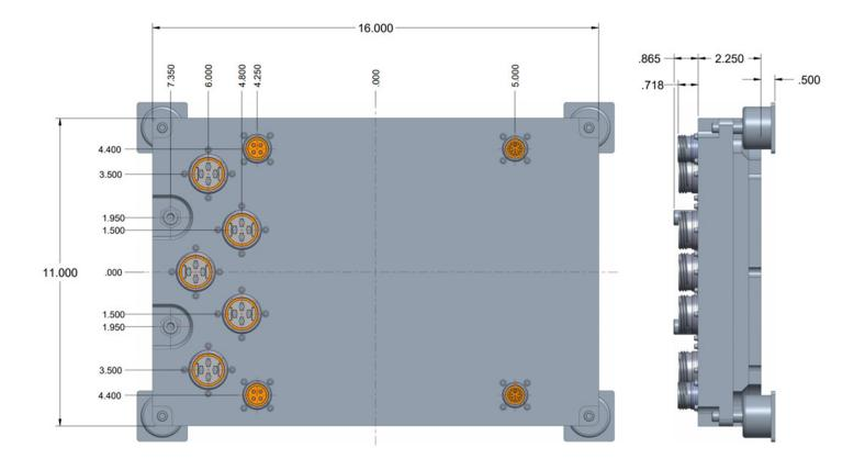
L2/L3 Managed Liquid Cooled Rugged Ethernet Switch
