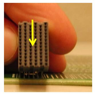
Figure 2. Back row of the DC connector compliant pins in the PTH.
