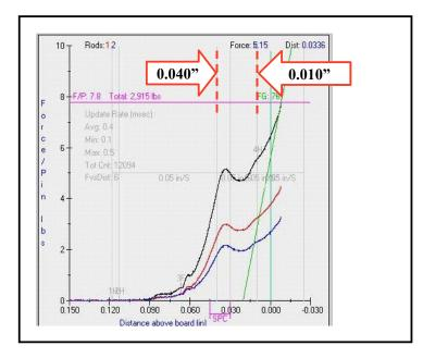
Figure A-12. Force vs. Distance Graph showing the "Max Force Per Pin" zone.
