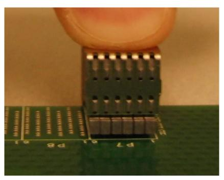
Step 7. Check for any bent pins protruding from under the connector assembly (see Figure 6).
