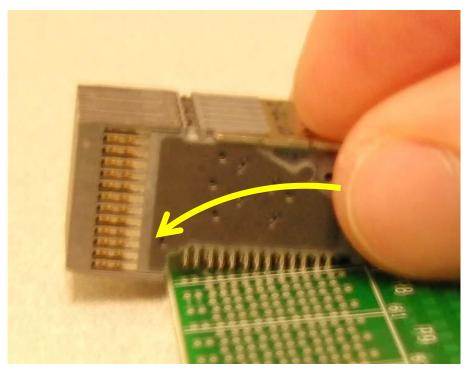
Figure 4. Side view: Roll connector toward board edge placing the remaining rows of compliant pins.
