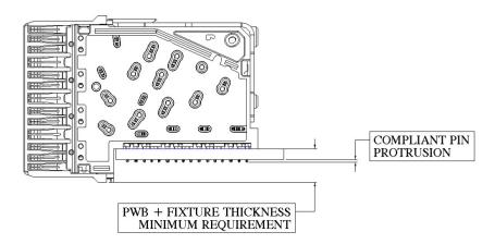
Figure A-9. Detail of PWB + Fixture thickness requirements and compliant pin protrusion of XCede HD, XCede HD PLUS & XCede HD2 Daughter Card connectors.
