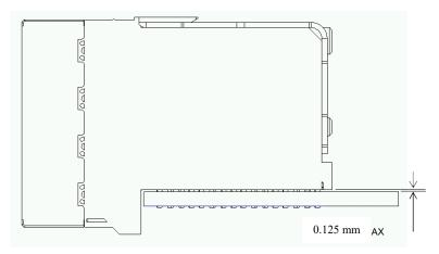
Figure 9. 0.125 mm maximum height off board surface
