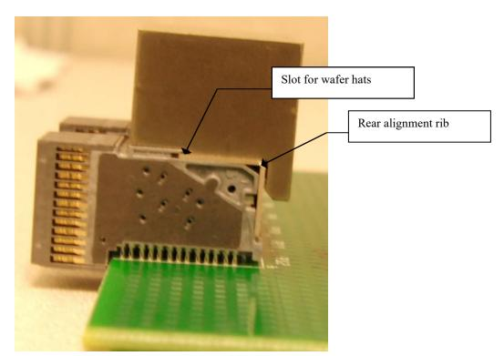
Figure 9. Clearance slot for wafer "retention hats" and rear alignment rib.
