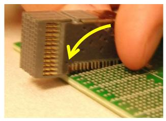
Figure 3. With the back row entirely placed, roll connector toward board edge placing the remaining rows of compliant pins.
