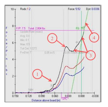
Figure A-10. Typical Force vs. Distance Curve of MEP-12T press for XCede HD, XCede HD PLUS & XCede HD2 connectors.
