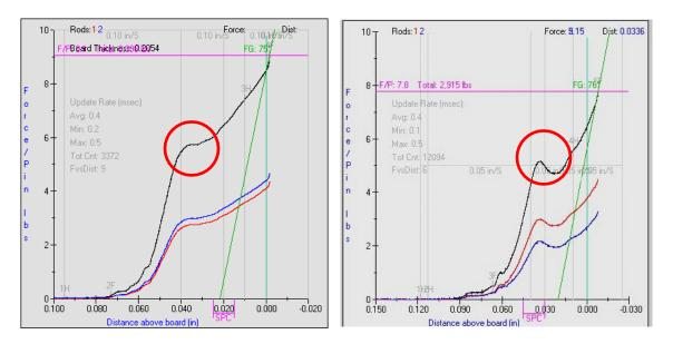
Figure A-11. XCede HD &XCede HD PLUS pressing Force vs. Distance Graph showing two shapes of the knee area utilizing an MEP-12T press.
