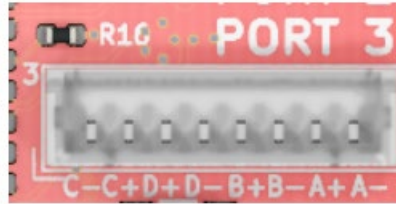
Ethernet port pinout
