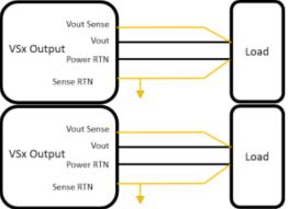
Figure 4: M4054 Sense line connection
