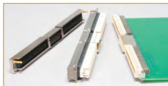
Ruggedized VME64x backplane (left), and module adapter (center) and a typical COTS VME64x circuit board (right).
