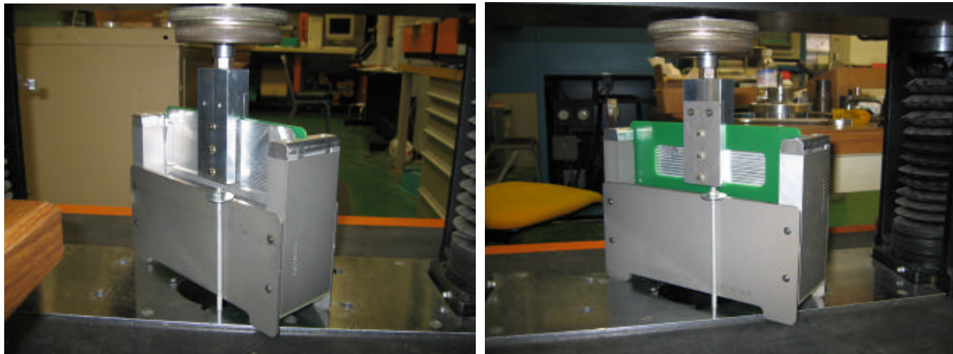
FIGURE 1. INITIAL MATING FORCE TEST SET-UP.
