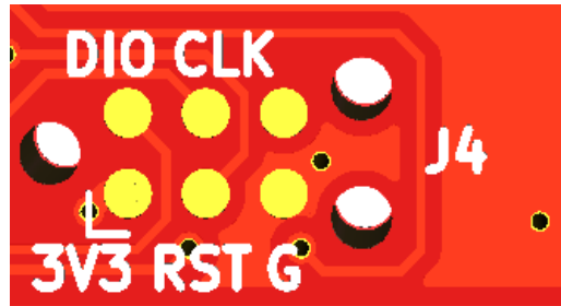
Figure 10: SWD programming header pinout
