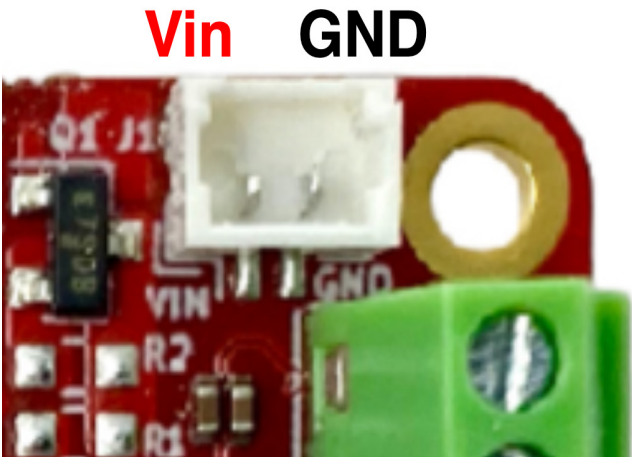
Figure 5: Voltage input header pinout
