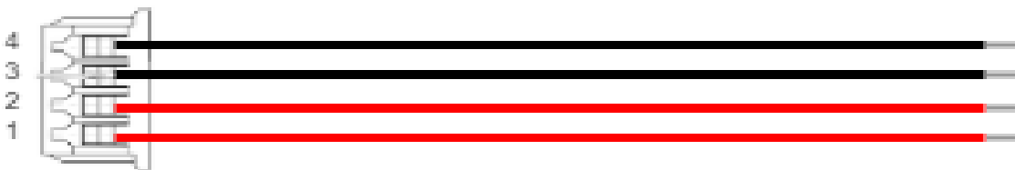
Figure 3: Voltage input cable pinout (red = V+, black = GND)
