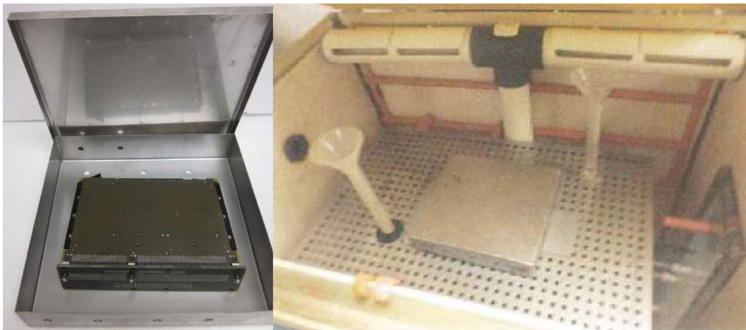
Figure 8: Salt Fog with SO 2 test set-up
