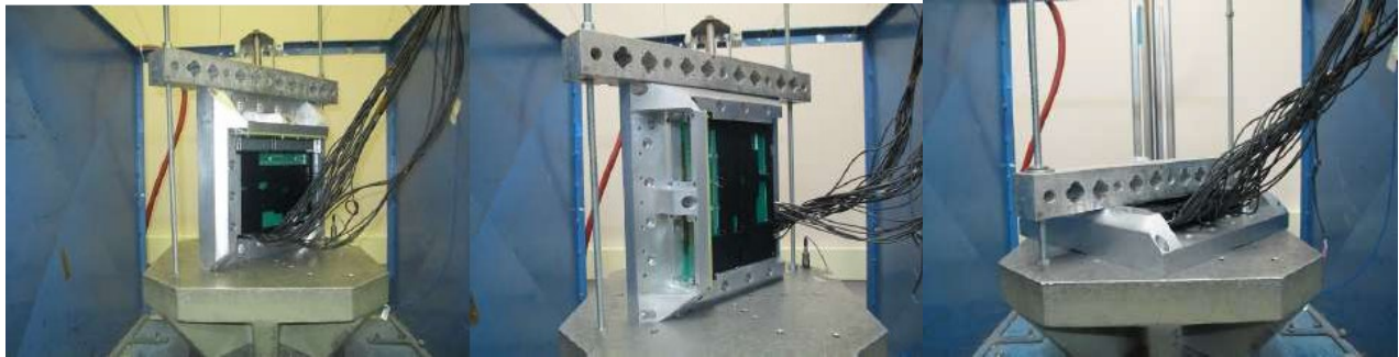
Figure 7: Mechanical Shock test set-up
