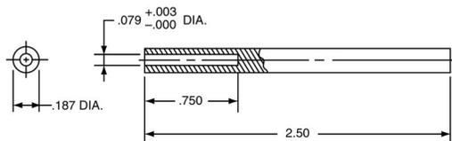
CONTACT INSERTION INTO CONNECTOR
