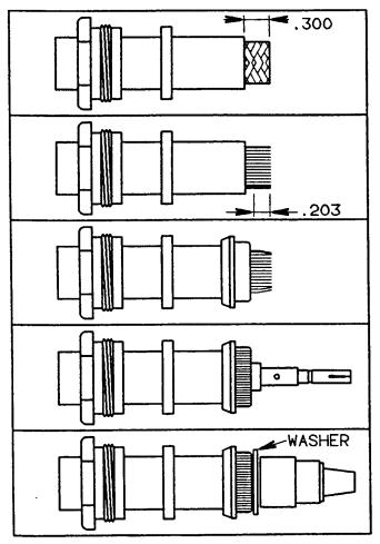
SLIDE NUT AND SEAL OVER CABLE WITH FLAT SIDE OF SEAL AGAINST NUT. CUT JACKET TO .300"
