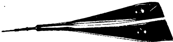
Figure 5. Gripping Standard Size 20 Contacts
